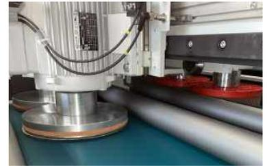
Four rotating discs with full-width oscillation for uniform 360° processing
