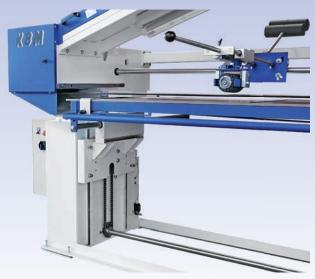
Table height adjustment by means of flat guide on both sides via chain and gear motor.
