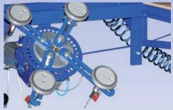
The workpieces are held in place by vacuum suction cups. The handling mechanism is activated by a foot switch.
