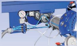
The workpiece is positioned relative to the grinding belt via three shafts, which are pneumatically locked by the locking disc (infinitely) and/or via grid holes.
