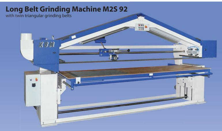
Long Belt Grinding Machine M2S 92, basic configuration, with a flat machine table and twin offset. Ideal for panels, profiles and small housings. Supplied as standard with variable belt speed, belt width either 100 or 150 mm.
