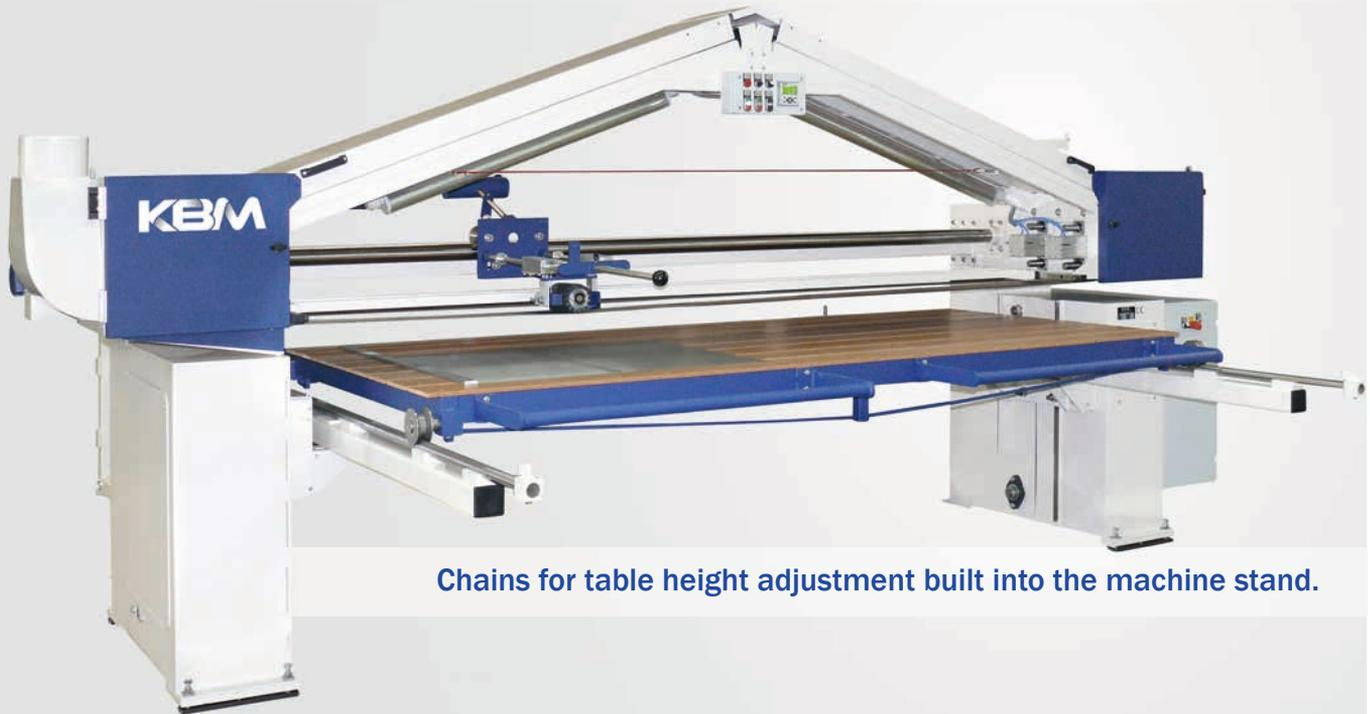
Chains for table height adjustment built into the machine stand.
