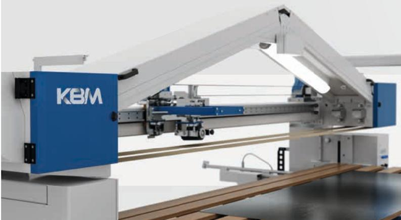
The grinding unit is mounted on a stable guide and is driven via a timing belt. The contact roller automatically moves between the two grinding belts, depending on the selected grinding program.
