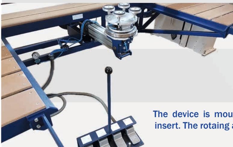
DUO table as 3-axis table with integrated 3D handling device for pivoting and rotating the workpieces.
