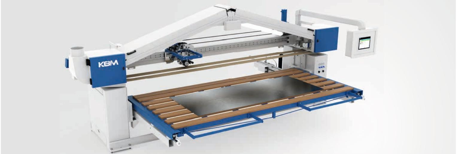
This automatic machine is controlled by a Siemens PLC. The machine has various grinding programs for different grinding applications.
