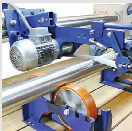
Tube grinding assembly consisting of a lateral grinding belt, with drive and idle rollers.
