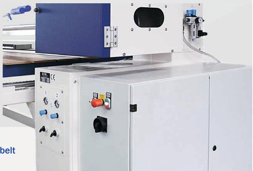
Right-hand machine stand with offset, switches and pressure regulator for pneumatic belt tensioning. Operated from the front.
