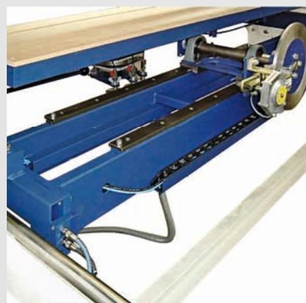
3D handling unit can be moved on guides from the centre to the right side of the table.
