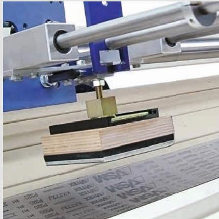
Grinding pad with ball-type quick fastener.
