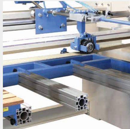
Aluminium cantilever arms to hold box-shaped workpieces.
