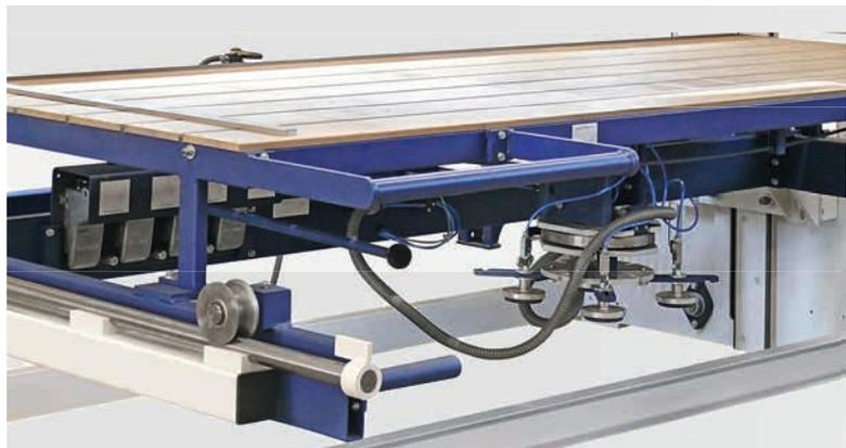
Flat machine table as an add-on table. The 3D handling device pivoted downwards and stored underneath.
