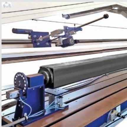
Pneumatically operated workpiece clamping and turning device mounted on the machine table.
